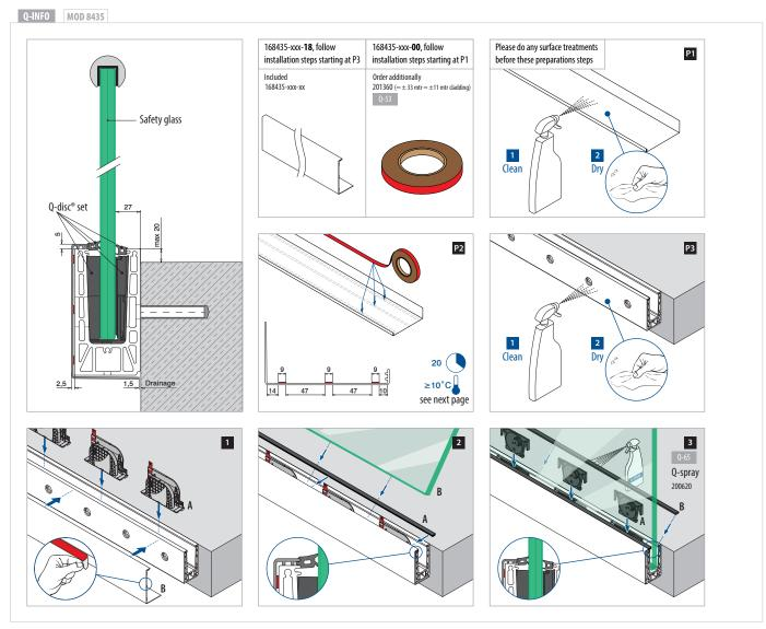
EASY GLASS® PRIME FASCIA CLADDING - adhesive tape mounting instructions - Alternative mounting option
