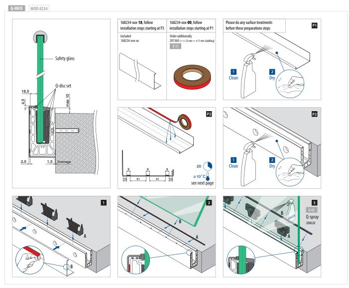
EASY GLASS® SMART FASCIA CLADDING - adhesive tape mounting instructions - Alternative mounting option
